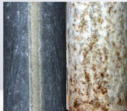
Magnelis® ZM310 welded and re-protected Post-galvanised welded
