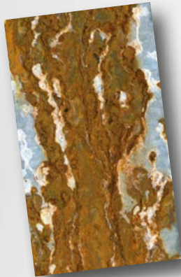
Hot dip galvanised 20 \mu\text{m} after 6 weeks
