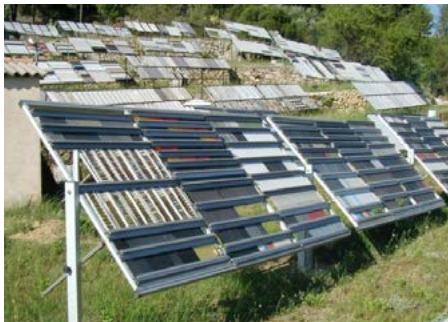
Granite® HDX test panels at the Station d'Essais de Vieillessement Naturel (SEVN) in Sanary-sur-Mer, France. Photograph: © ArcelorMittal Global R&D
